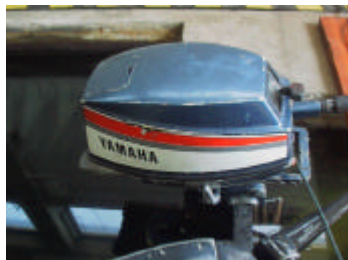
Figure 66 - Motor 3, a 3.6 hp Yamaha
